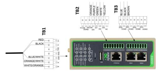
To program RS485 port 2, connect to controller via USB or ethernet connection and the DSE Configuration Suite software. From left side pane navigate to G8600 Configuration – Communications – RS485 Ports. Update Port 2 settings to the below:
